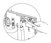
2 - Screw the connection (female) on the entrance (male) using the supplied gasket, keeping it tight.
