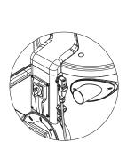
2 - Connect the plug on the Autocleaner and close the safety catch.
